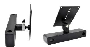
Headrest holder solid aluminium - black powder coated, incl. small ball mounting device with straight flange, black/silver anodized aluminium and height adjustable VESA-plate: 85 x 115 x 4mm, hole pitch 75 x 75 mm
